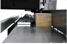
The feeding device has 13 wear resistant wheels. Every wheel is separately spring-loaded.
